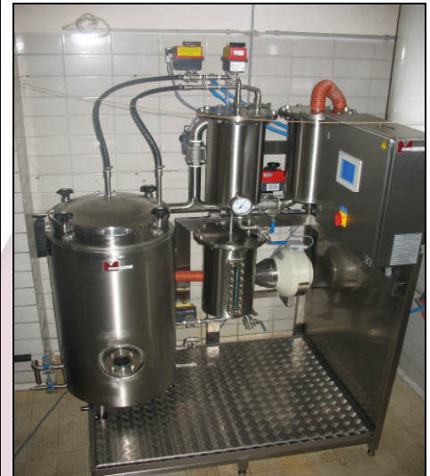
BDU-1370-50 Bone Degreasing Unit with DCM-recycling and bone drying modules. Degreasing chamber size: 500mm AD x 900mm
