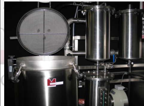
BDU 1370-50 with process chamber with patented screen-shower (left), DCM recycling system (middle) and dryer (below right).
