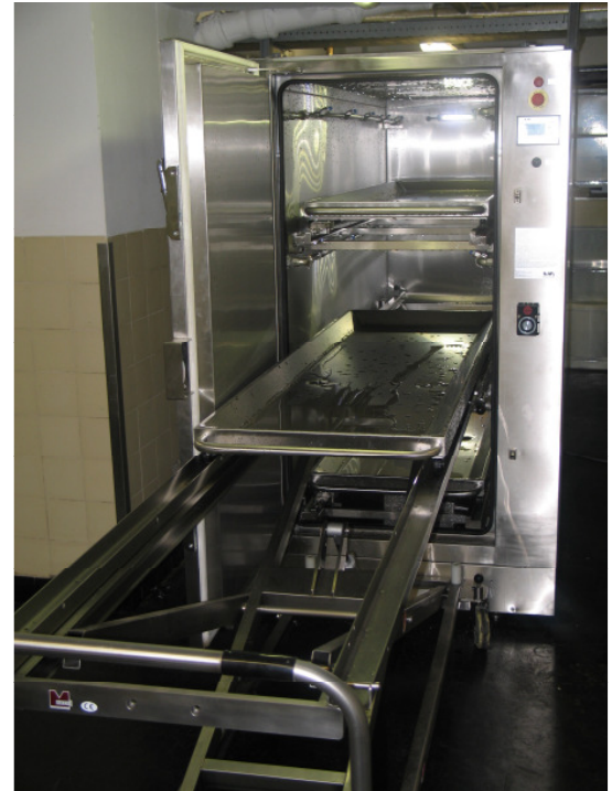
Automatic loading / unloading of the SprayCon unit
